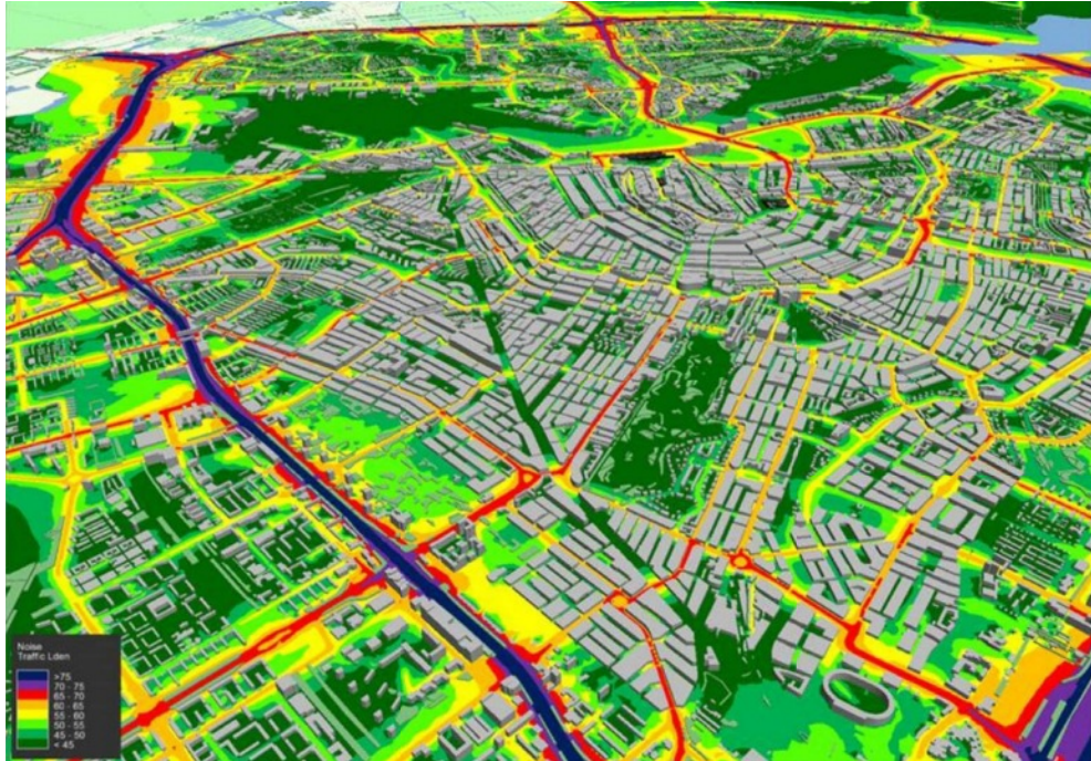
Figure 4. 3D representation of traffic noise in Amsterdam (Lden) in the Local Digital Twin
